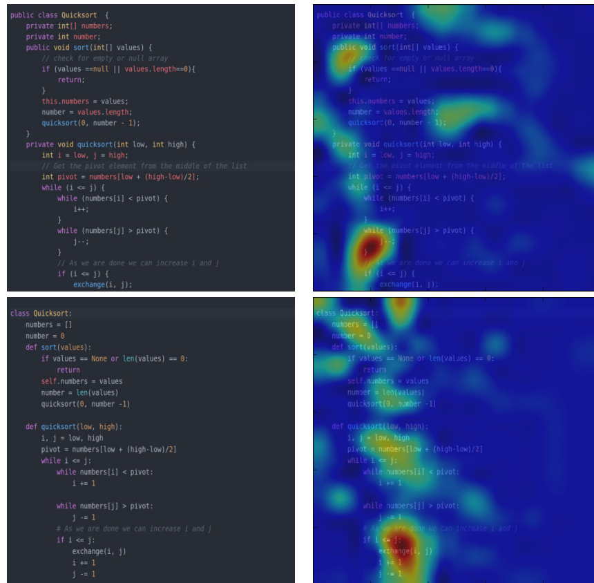
Figure 2: CAM results on correctly predicted Java (top) and Python (bottom) code image frames, of the Quicksort algorithm. The left column shows the normal test image. The right column shows the CAM results overlaid on the test image.
